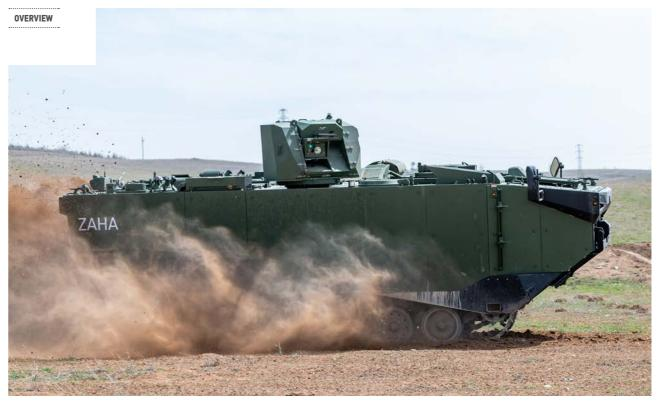
During the beach-landing phase of amphibious operations, these vehicles are launched from amphibious assault ships and are able to rapidly cover the distance between the vessel and the shore, allowing marine units to land under armour protection. MAV have all the features and capabilities of both a military land vehicle and a military marine vessel, by balancing the land and sea requirements. This dual role by definition, vehicle offers high performance both on land and water operations.
